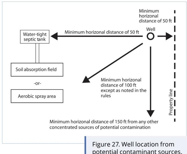
In addition, every effort must be made to locate a new well where it will not be vulnerable to flooding. Floods can cause the contaminants from the surface to seep down the outside of the well casing and pollute the aquifer.
