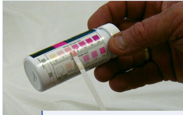
Figure 50. Home water testing kits typically rely on a color change on a test strip to determine the concentration of a contaminant.
