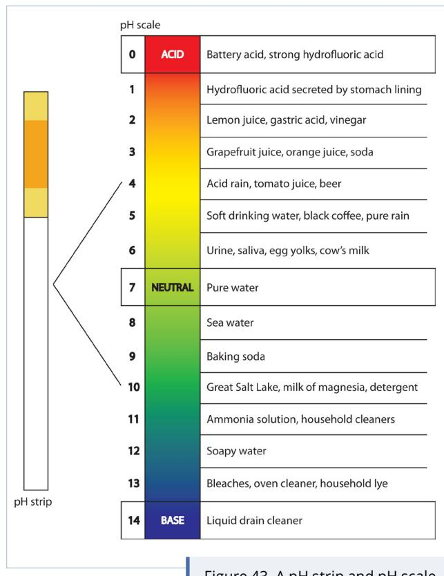
Figure 43. A pH strip and pH scale.
