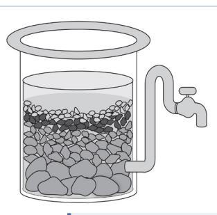
Figure 53. A simple filtration system.
