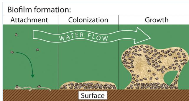
Figure 47. Biofilms form from slime bacteria that feed on iron, manganese, and/or nitrate.
