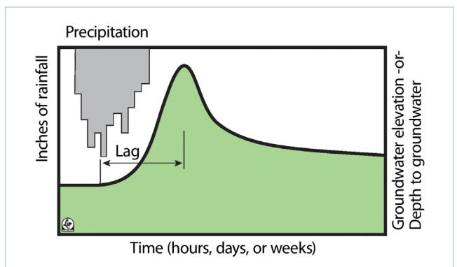
Figure 8. A hydrograph shows the changes in water-table elevation over time.
