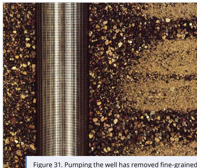
Figure 31. Pumping the well has removed fine-grained sediment from around the well screen. Reprinted by permission of Johnson Screens, a Weatherford Company.
