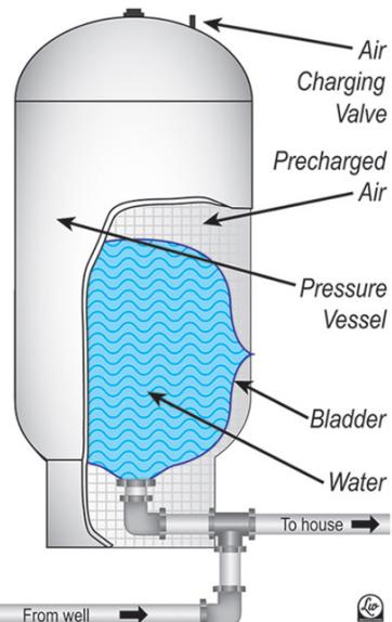
Figure 33. Pressure tank for a private well system. (Source: Gary Hix)
