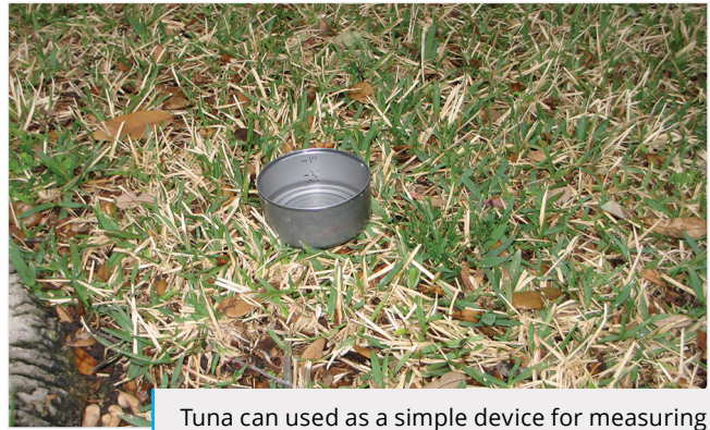
Tuna can used as a simple device for measuring precipitation rate in an irrigation evaluation.
