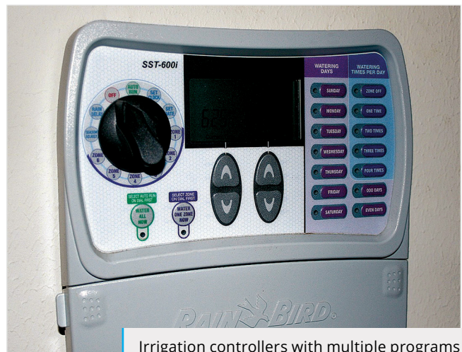
Irrigation controllers with multiple programs allow waterings to be broken up into several shorter cycles for each zone.
