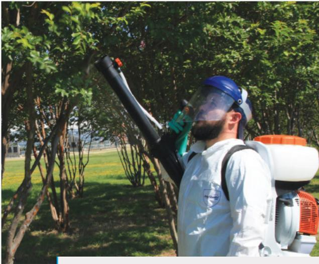
Figure 4. Backpack mist blower being used by a pest control company employee to treat mosquito resting sites with a long-lasting insecticide.
