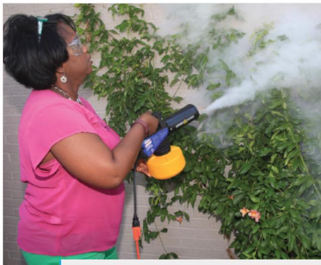
Figure 3. Small thermal fogger producing a dense fog to kill mosquitoes resting in backyard vegetation and shrubs. Fogs work best when applied in the evening or when there is little wind.
